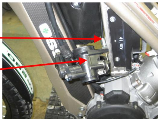
Push the air filter up through the air box pass the ECU and out. Optional, but recommended is to place a clean rag in the manifold.
