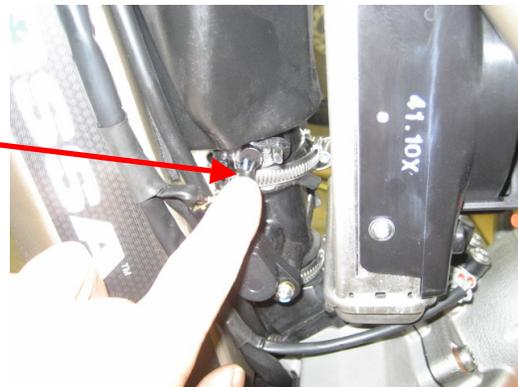
Air filter temp. sensor receiver and tabs. Tabs will be used for installation to snap sensor into position.
