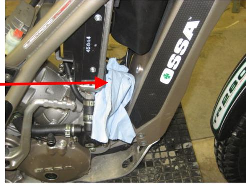
To reinstall, push clean and oiled air filter through the air box with the temperature sensor hole pointing to the left. With the throttle body out of the way you will be able to pull the air filter through from the bottom. Pull the left side through with the sensor hole first, then slide the right side through, there are pull tabs to accomplish this.
