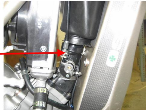
Fit the temperature sensor into the air filter receiver using the two tabs on the filter to guide it on. Grab one tab lightly with your fingers or pliers and push the sensor in, you will feel the tab snap into position on the sensor. Repeat the other side of the sensor.
