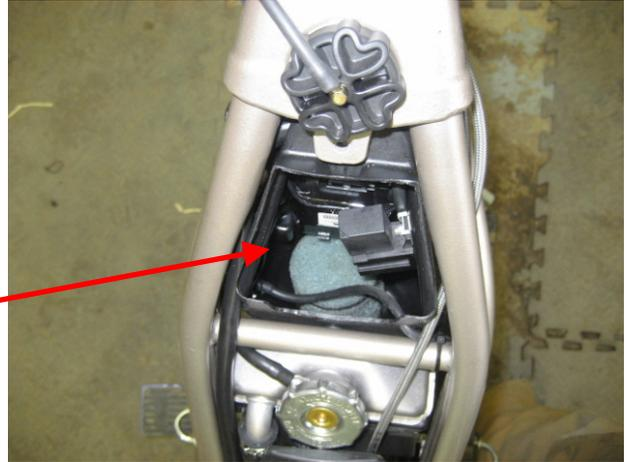
Remove the fan relay and set to right side of air box.
